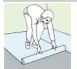
1. Check the evenness of the floor of the room. For this purpose use an approx. 2m long straight lath. If the floor deviation is more than 2mm, we suggest that you level the floor. In the case of a cement floor the moisture content of the floor should not be higher than 2 %.
