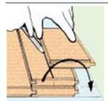
7. Fitting is done with a piece of wood used for hammering the parquet pieces together.
